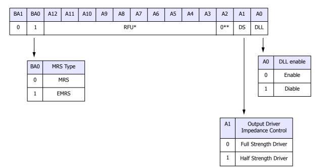
\* All bits in RFU address fields must be programmed to Zero, all other states are reserved for future usage \*\* This part do not support /QFC function, A2 must be programmed to Zero.
